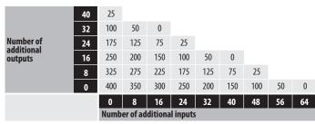
Max. residual current values (in mA) for FX3U-48M $\Box$ -E $\Box$  through FX3U-128M $\Box$ -E $\Box$  for the permissible configuration
