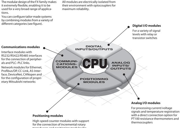
transducers and positioning modules for servo and stepping motor drives
