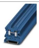
Feed-through terminal block, connection method: Screw connection, number of connections: 2, cross section:0.14 mm² - 4 mm², AWG: 26 - 12, width: 5.2 mm, height: 46.9 mm, color: blue, mounting type: NS 35/7,5, NS 35/15
