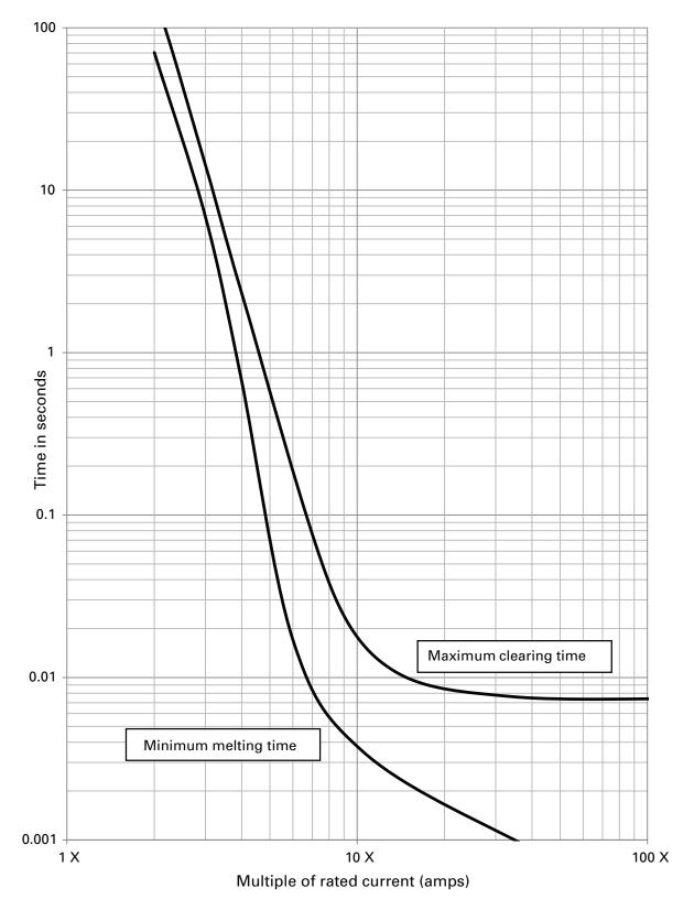
For 100 to 150 amp fuses supplied via DC rectifier @ 500 Vdc and time constant (L/R) 2 ms ± 0.5 ms
