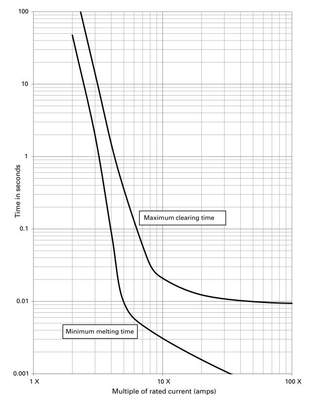
For 125 to 150 amp fuses supplied via DC rectifier @ 500 Vdc and time constant (L/R) 2 ms  $\pm$  0.5 ms
