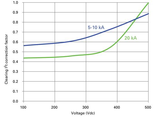
\* Correction factor applies to I<sup>2</sup>t clearing at 20 kA in the catalog number table on page 2.
