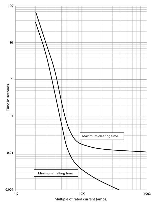
For 200 to 400 amp fuses supplied via DC rectifier @ 500 Vdc and time constant (L/R) 2 ms ± 0.5 ms
