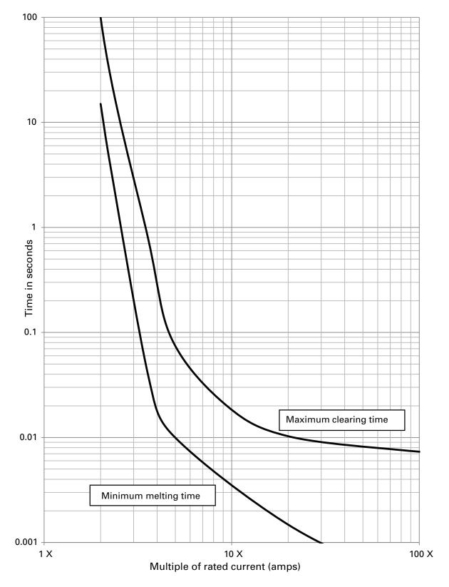
For 175 to 250 amp fuses supplied via DC rectifier @ 500 Vdc and time constant (L/R) 2 ms  $\pm$  0.5 ms
