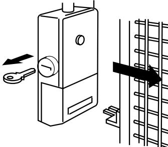
Guard door can now be opened. The key can be withdrawn for use as a personnel key to prevent entrapment within the enclosure.
