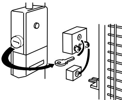
Key can be held by operator or used in an exchange system.
