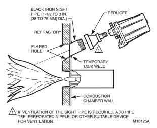
Fig. 5. Typical mounting of C7061.
