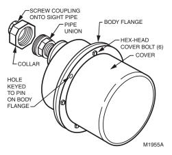
Fig. 9. Mounting a C7061F Detector.
