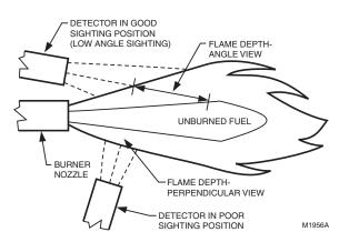
Fig. 3. Detector sighting angle.
