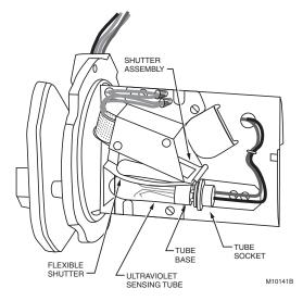
Fig. 12. Replacing ultraviolet radiation sensing tube.
