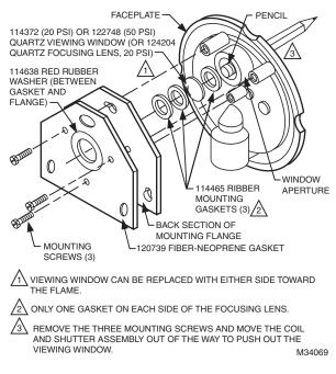
Fig. 14. Replacing quartz viewing window or focusing lens.
