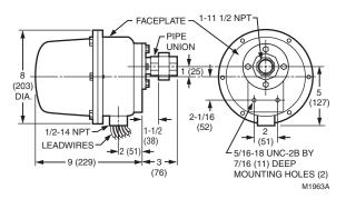
Fig. 2. Dimensions of C7061F in Inches. (mm).
