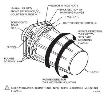
Fig. 8. Mounting C7061A Detector.
