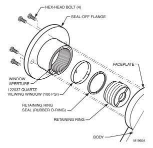
Fig. 15. Replacing quartz viewing window on C7061F.
