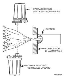
Fig. 6. Vertical mounting of C7061A.
