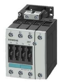
CONTACTOR, AC-3 18.5 KW,400V, AC 230 V, 50 HZ 4-POLE, 2 NO + 2 NC, SIZE S2, SCREW CONNECTION
