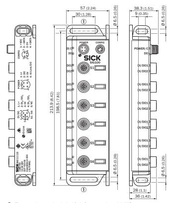
$\bigcirc$  Elongated mounting hole (4 x), for mounting with M6 screw
