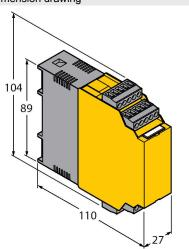
Trip amplifier; 1-channel; input 0/4... 20 mA or 0/2...10 V; supply of 2- or 3-wire transmitters/sensors; limit value adjustment via teach button; three relay outputs with one NO contact each; removable terminal blocks; 27 mm wide; universal voltage supply 20...250 VUC; further Limit value indicators are described in our "Interface Technology" catalog.
