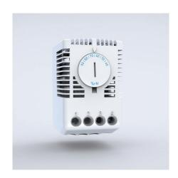
**Description:** Mechanical hygrostat designed to control heaters when the pre-set or fixed relative humidity is exceeded. The relative humidity must be kept above the dew point to prevent condensation and corrosion inside the enclosure. Mounting clip for 35 mm DIN rail (EN 60715).
