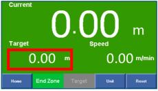
The two indicators will turn either green or red depending on the state of the target and endzone. In the screenshot below the target is grey since no target has been set. Once the end zone is reached, this will turn to red to indicate that the relays have changed states, and then once the target is reached, this will turn red and the endzone will return to green to indicate that the target has changed states but the endzone has returned to its original state.
