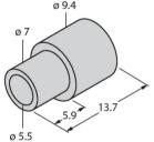
Spacer sleeves for rear mounting of RI-QR14, 2 pcs. per bag
