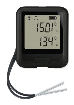
The sensor is IEEE 802.11bgn\* (2.4GHz) compliant, supports WEP, WPA/WPA2 encryption and enterprise networks (PEAP, TTLS, FAST).
