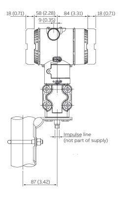
Figure 3 Standard static transmitter with barrel housing - vertical flanges
