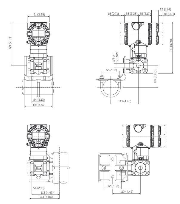
$Figure \, 5 \quad Transmitter \, with \, Kynar \, flanges \, on \, bracket \, for \, vertical \, or \, horizontal \, 60 \, mm. \, (2 \, in.) \, pipe \, mounting$
