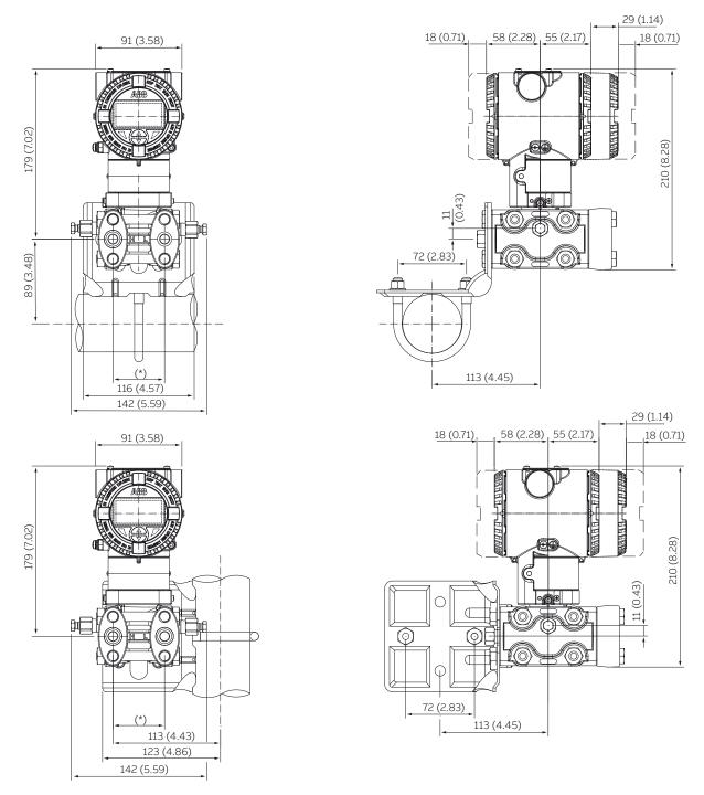
Figure 4 Transmitter on bracket for vertical or horizontal 60 mm. (2 in.) pipe mounting
