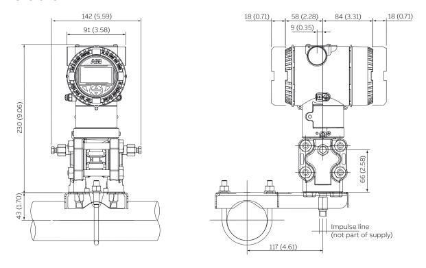
Figure 8 Transmitter with vertical flanges on bracket for vertical or horizontal 60 mm. (2 in.) pipe mounting
