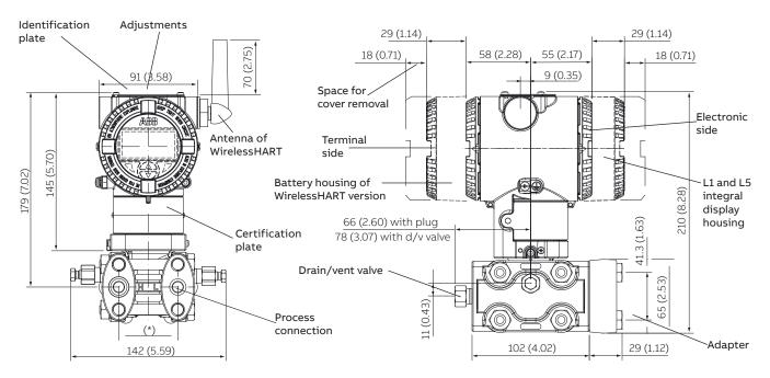
(\*) 54 (2.13) mm (in) on 1/4 – 18 NPT process flange; 51 (2.01), 54 (2.13) or 57 (2.24) mm (in) according to 1/2 – 14 NPT adapters fitting 54 (2.13) mm (in) with negative side provided with a removable filter for gauge measurement (version 266DSHxP)
