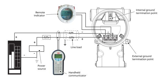
HART hand-held communicator may be connected at any wiring termination point in the loop, providing the minimum resistance is 250 ohm. If this is less than 250 ohm, additional resistance should be added to allow communications. Maximum voltage drop on external remote indicator is 0.7 V DC.
