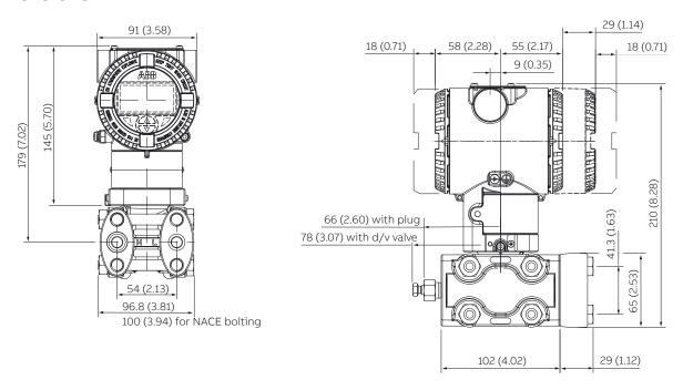
Figure 2 High static transmitter with barrel housing - horizontal flanges
