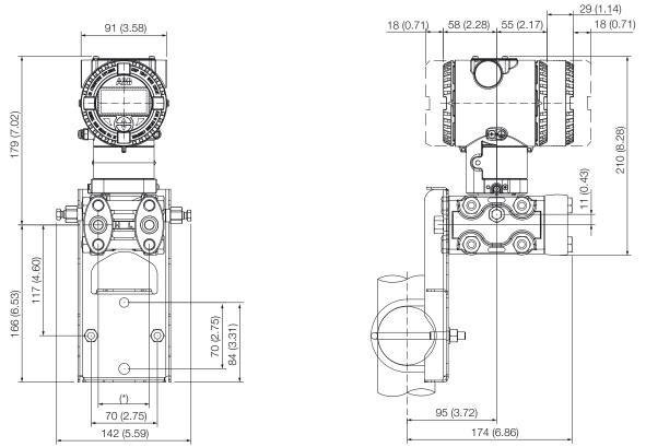
$Figure \ 7 \quad Transmitter \ with \ horizontal \ flanges \ on \ flat \ bracket \ for \ vertical \ or \ horizontal \ 60 \ mm. \ (2 \ in.) \ pipe \ mounting$
