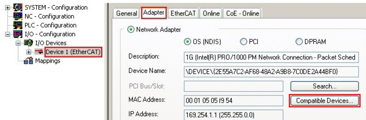
Fig. 32: EtherCAT device properties (TwinCAT 2): click on “Compatible Devices...” of tab “Adapter”
