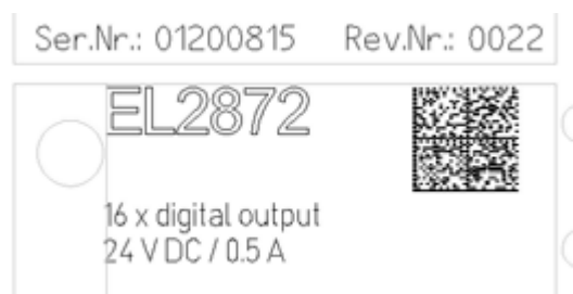
Fig. 1: EL2872 with revision 0022 and serial number 01200815
