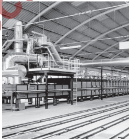
Roller hearth kiln in the ceramics industry.
