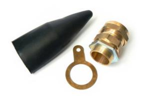
The Termination Technology range of CW Brass cable glands suitable for termination steel wire armour (SWA) cable. Suitable for outdoor application, all packs supplied complete with glands, PVC shrouds, galv locknuts and brass earth tags. Smaller sizes up to and including CW32PK are supplied in packs of 2, CW40PK and above are supplied in packs of 1. BW indoor gland packs also available as well as LSF versions of both ranges.
