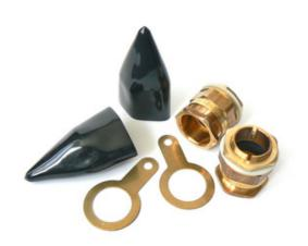
The Termination Technology range of CXT Brass cable glands suitable for use with all types of screened flexible wire braid and wire braid armour cables. Suitable for outdoor application, all packs supplied complete with glands, PVC shrouds, galv locknuts and brass earth tags. Smaller sizes up to and including CXT32PK are supplied in packs of 2, CXT40PK and above are supplied in packs of 1.
