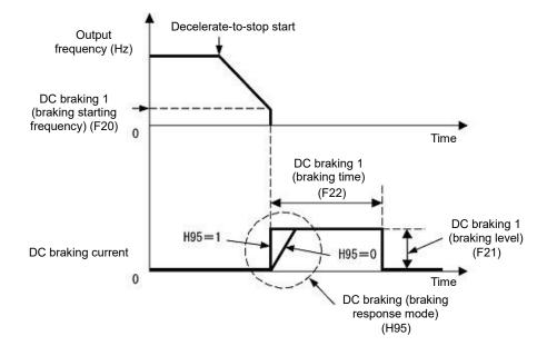
Tip It is also possible to input DC braking command "DCBRK" by using an external digital input signal as the terminal command. As long as the DCBRK is ON, the inverter performs DC braking, regardless of the braking time specified by F22.
