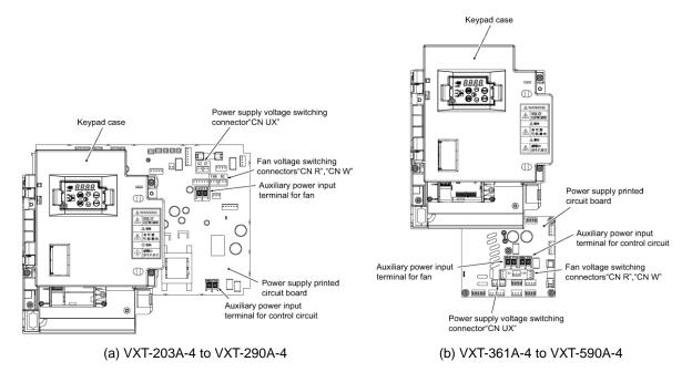
Figure 2.2-23 Switching Connector Positions
