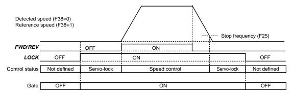
Figure 5.3-21 Typical Control Sequence of servo lock
