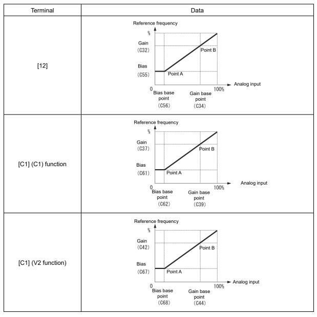
(Example) In order to allocate for the range of 0 to 100% to the range of 1 to 5 V at terminal [12], set as follows.
