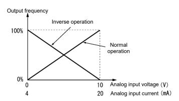
Tip The normal/inverse switching operation is useful for air-conditioners that require switching between cooling and heating. In cooling, the <u>speed</u> of the fan motor <u>(output frequency of the inverter)</u> is increased to <u>lower the temperature</u>. In heating, the <u>speed</u> of the fan motor <u>(output frequency of the inverter)</u> is reduced to <u>lower the temperature</u>. This switching is realized by the IVS.
