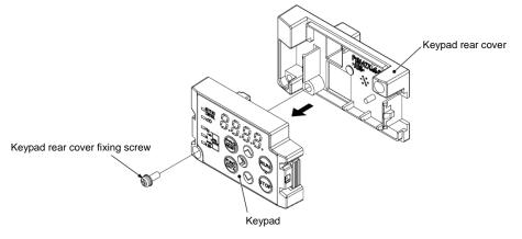
Figure 2.3-5 Attachment of the Keypad
