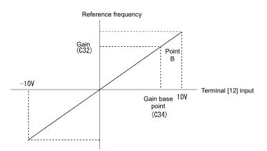
Note • When bias (F18) and bias reference point (C50) is set to arbitrary value (A1 point, A2 point, and A3 point, etc.), as shown in the diagram below, it is determined by the bias value (F18).
