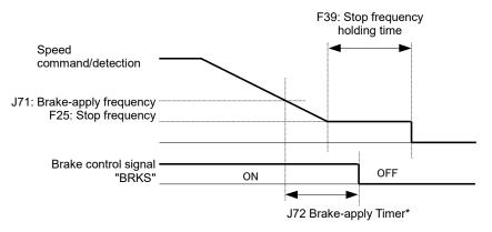
\* If inverter output was turned off before the timer counts up, then the brake is applied.
