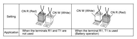
Figure 5.3-9 Fan power supply switching
