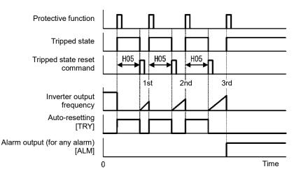
• The auto-reset operation can be monitored from the external equipment by assigning the digital output signal TRY to any of the programmable, output terminals [Y1], [Y2] or [30A/B/C] by setting E20, E21 or E27 respectively (data = 26).
