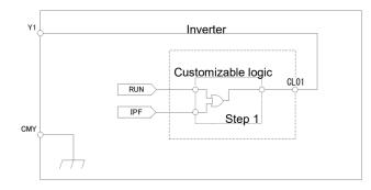
To configure this customizable logic, set the function codes as follows. (Timer selection) and (Timer setting) do not need to be modified if no change is made.
