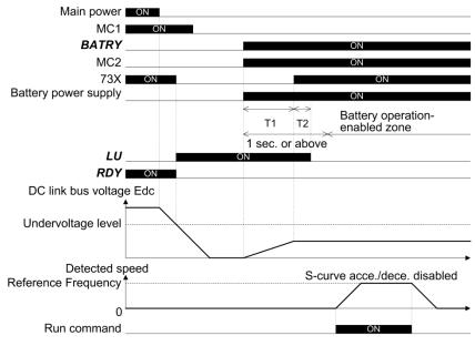
Figure 5.3-10 Battery operation timing chart
