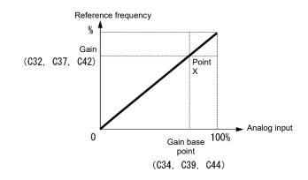
Note To input bipolar analog voltage (0 to ±10 VDC) to terminal [12], set C35 data to "0." Setting C35 data to "1" enables only the voltage range from 0 to +10 VDC and interprets the negative polarity input from 0 to -10 VDC as 0 V.
