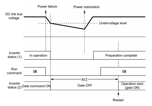
Factory default: At the factory default state, setting is performed so that it is appropriate to the standard motor (refer to "5.2.3 Factory default value per applicable electric motor capacitance"). Basically, there is no need to modify the default setting. However, when problems occur due to the long holding time or decrease in flow rate of pump becomes significant, change to about half of the standard value and make sure that alarm etc. will not occur.
