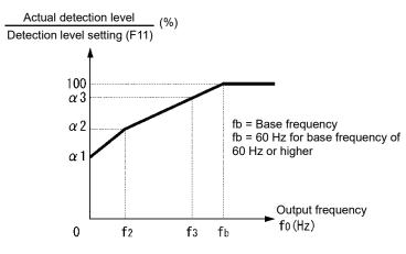
Figure 5.3-3 Characteristics diagram of motor cooling system
