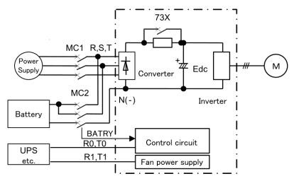
Figure 5.3-8 Connection diagram example (VXT-203A-4 or above)
