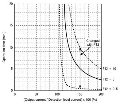
Figure 5.3-4 Example of current-operation time characteristics
