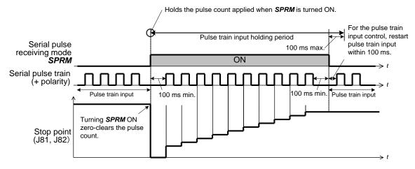
Figure 5.3-20 Switching the Input Mode between the Pulse Train Input and Serial Pulse Receiving Mode
