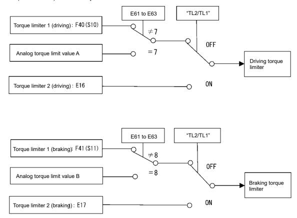
Note The torque limiter and current limiter are very similar in function. If both are activated concurrently, they may conflict with each other and cause hunting (undesirable oscillation of the system). Avoid concurrent activation of these limiters.
