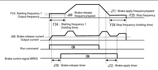
Figure 5.3-16 Operation time chart under v/f control
