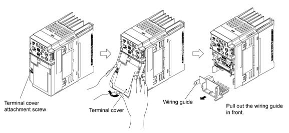
Figure 2.2-3 Removal of the Terminal Cover and the Wiring Guide (for VXT-6A-2)
