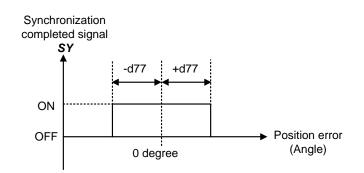
Figure 5.3-29 Synchronization Completion Detection Signal "SY"
