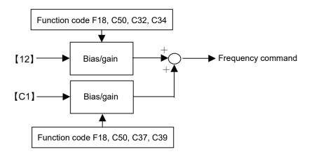
For single polarity (Terminal [12] (C35=1), Terminal [C1] (C1 function), Terminal [C1] (V2 function)
