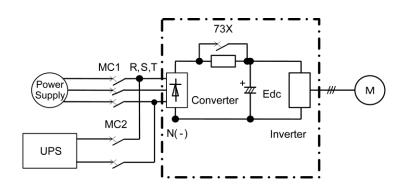
Figure 5.3-5 Connection diagram example (VXT-115A-2 or below, VXT-85A-4 or below, VXT-12A-1 or below)
