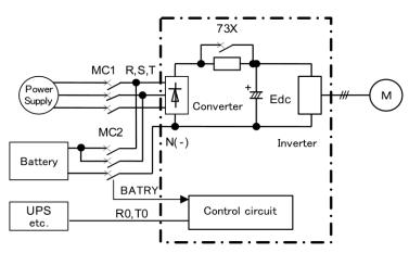
Figure 5.3-7 Connection diagram example (VXT-115A-2 or below, VXT-168A-4 or below)
