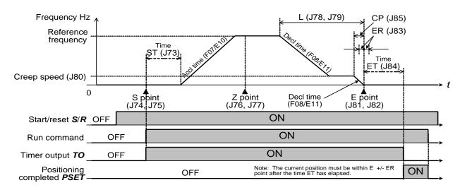
Figure 5.3-18 Positioning Control Behaviour
