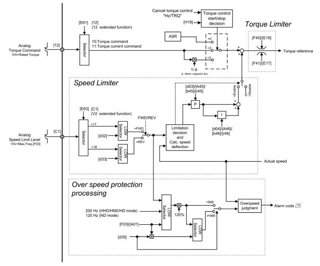
Figure 5.3-11 Block Diagram of Torque Control
