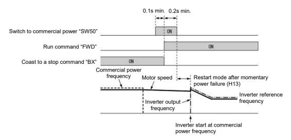
• When the motor speed decreases significantly during coast-to-stop (with the current limiter activated)
