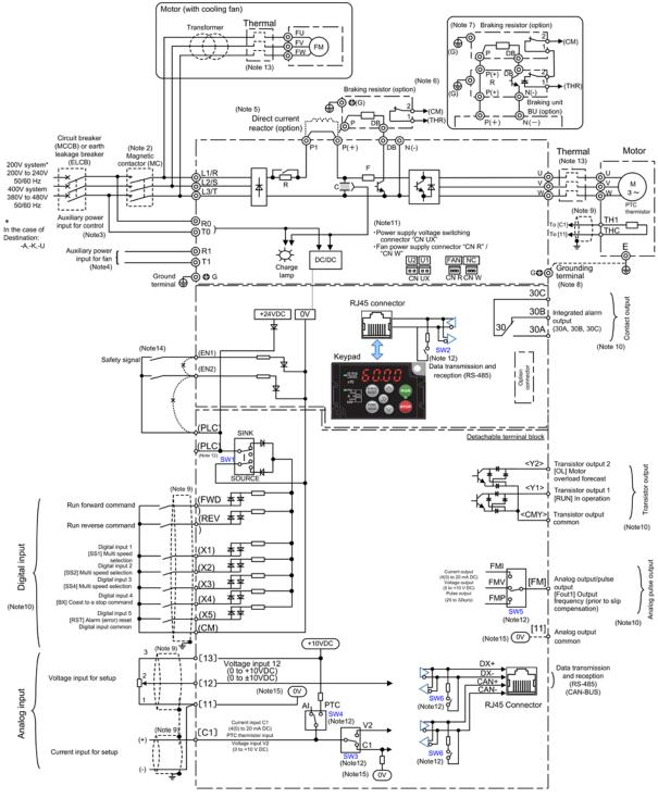
Figure 2.2-1 Standard model (with CAN)
