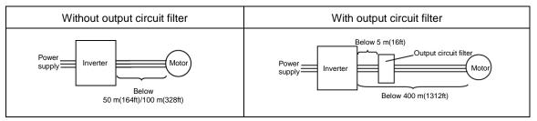
When the output circuit filter is used, the total wiring length should be below 400 m (1312ft) in case of using V/f control.
