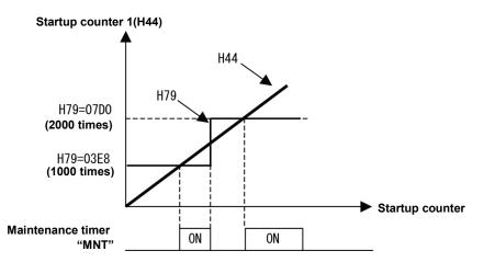
Note If the startup counter reaches the specified value, set a new value for the next maintenance in H79 and press the key to reset the output signal and restart counting.
