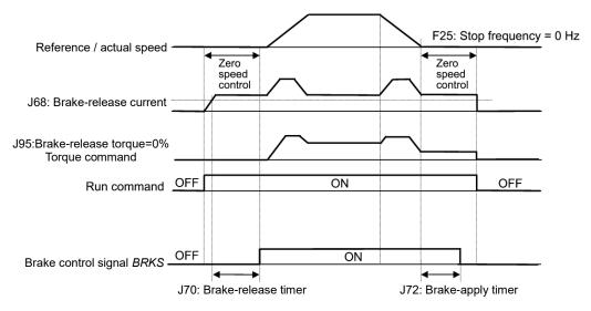
Figure 5.3-17 Operation time chart under vector control with speed sensor
