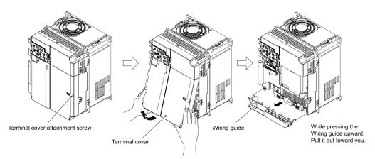
Figure 2.2-4 Removal of the Terminal Cover and the Wiring Guide (for VXT-69A-2)
