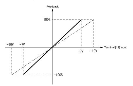
Example 2: When an external sensor has the output range of 0 to 10 VDC:
