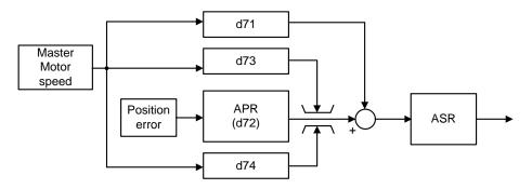
Figure 5.3-28 Operation of APR output limiter
