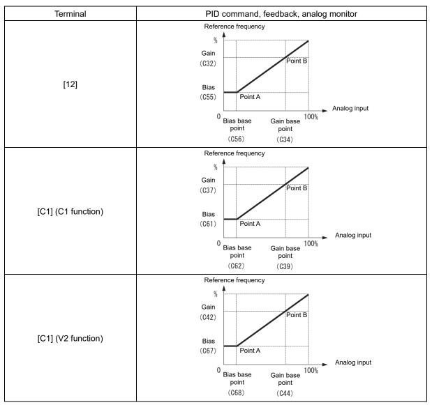
These are biases and bias base points used for PID command, PID feedback, frequency command 2 and analog monitor. For details, refer to the description of F01 and J01.
