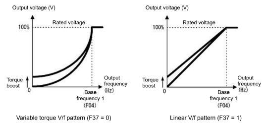
When the variable torque V/f pattern is selected (F37 = 0 or 3), the output voltage may be low at a low frequency zone, resulting in insufficient output torque, depending on the characteristics of the motor and load. In such a case, it is recommended to increase the output voltage at the low frequency zone using the non-linear V/f pattern.
