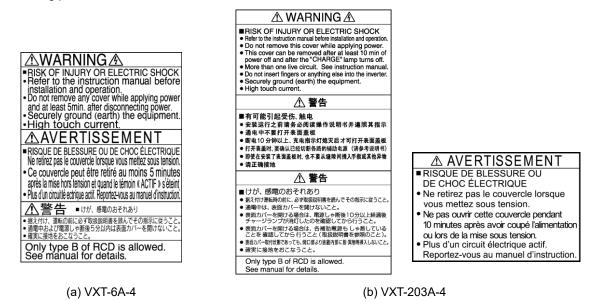
Figure 1.2-2 Warning Plates and Label
