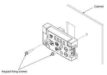
Figure 2.3-7 Attachment of the Keypad
