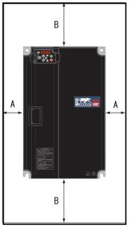
Figure 2.1-1 Installation Direction
