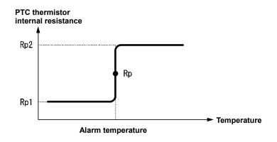
Suppose that the internal resistance of the PTC thermistor at the alarm temperature is Rp, the detection level (voltage)  $V_{v2}$  is calculated by the expression below. Set the value of  $V_{v2}$  to function code H27.
