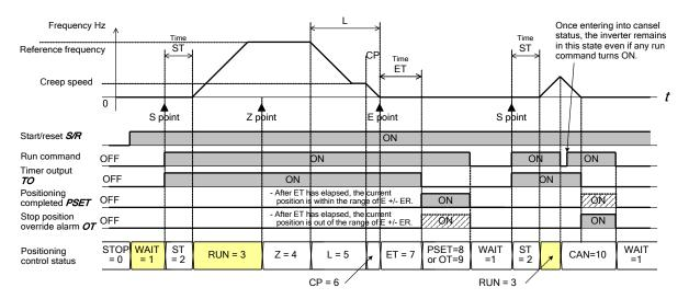
Figure 5.3-19 Positioning Control Status Transition Model
