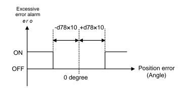
Figure 5.3-30 Excessive error alarm ero
