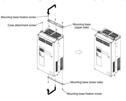
Figure 2.1-3 Method to Change the Mounting Base Positions
