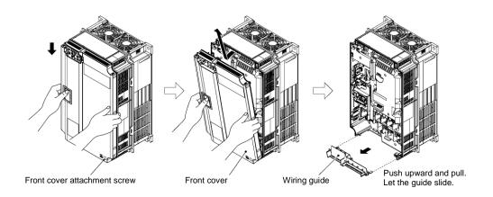
Figure 2.2-5 Removal of the Front Cover and the Wiring Guide (for VXT-72A-4)
