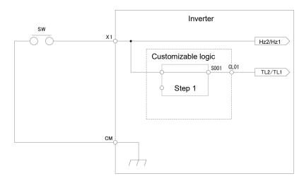
To configure this customizable logic, set the function codes as follows. (Timer selection) and (Timer setting) do not need to be modified if no change is made.
