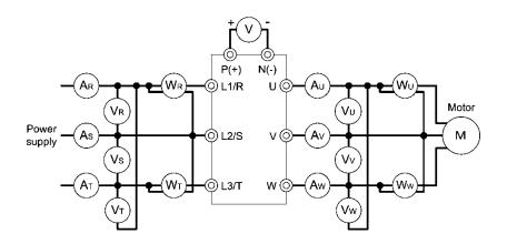
Figure 7.5-1 Connection of Meters
