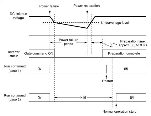
When allowable momentary power failure time (H16) is set to "999", momentary power failure restart is performed until DC link bus voltage decreases by momentary power failure restart allowance voltage (50 V for 200 V class, 100 V for 400 V class), however, if the voltage becomes at or below the momentary power failure allowance voltage, the state is judged as a power shut down. As a result, the inverter operates as powering ON again without performing momentary power failure restart operating.
