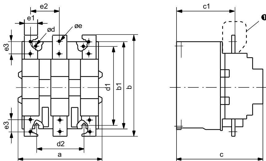
**Figure 42 - Mounting Position**
