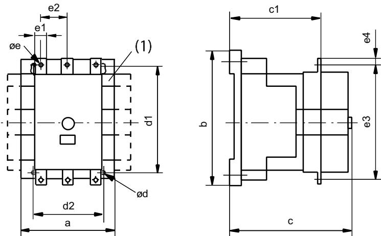
(1) Conventional DC coil contactors will have an additional auxiliary contact block that will add 13.5 mm to the "a" dimension on the right-hand side.
