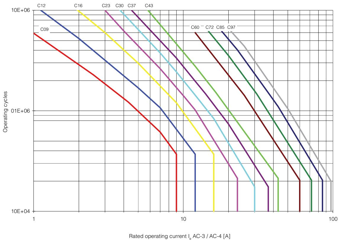
**Figure 12 - Heavy Duty Starting and Regular Short-time Operation**
