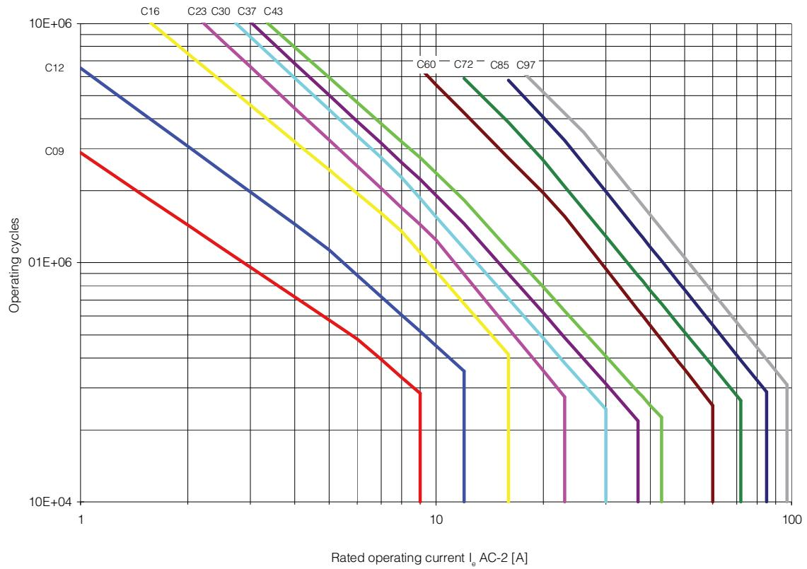
**Figure 7 - AC-3, Switching of squirrel-cage motors while starting;  $U_e = 230\ldots 400\ldots 460V$**
