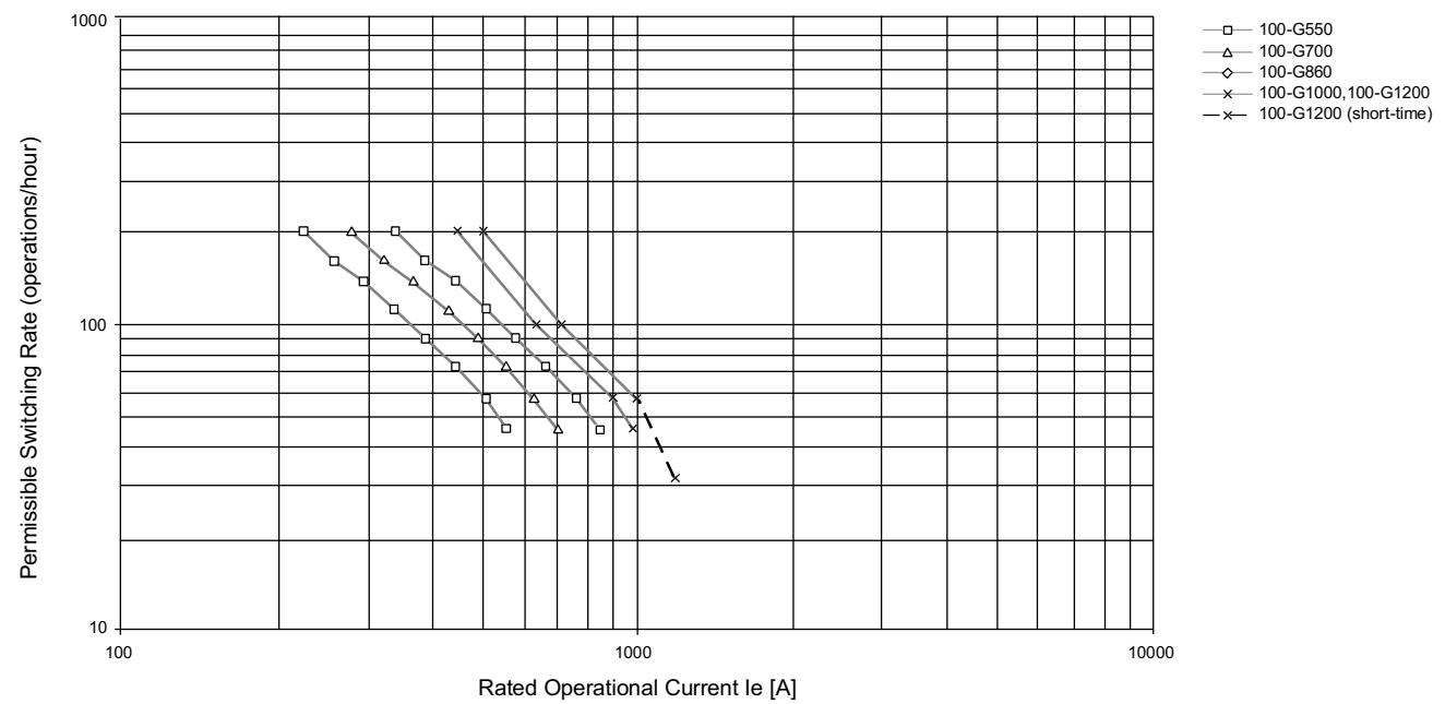
**Figure 40 - Switching of Starting Motors (AC-2, and AC4)  $U_z = 380\ldots460V$  AC; Starting Time  $t_{ed} = 1$  s, ( $< t_s$ )**
