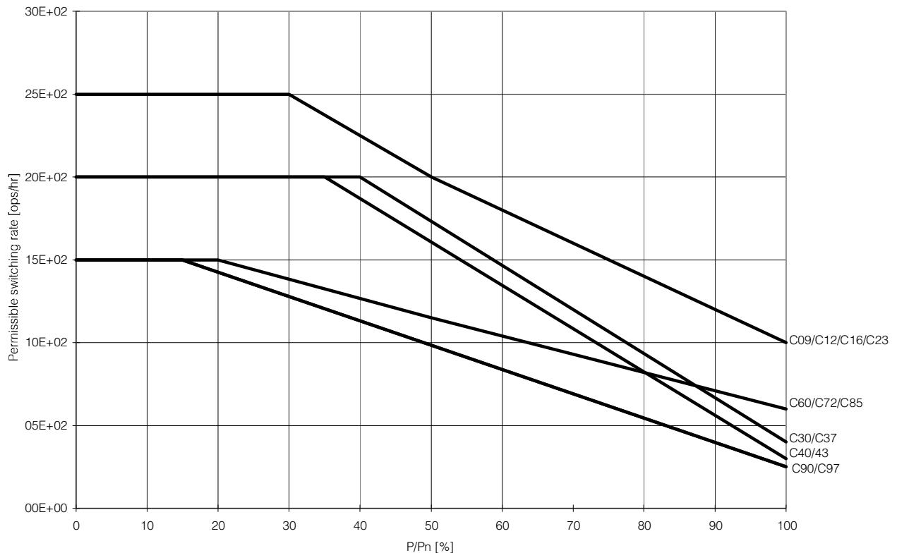
**Figure 14 - AC-2, Stepping of slip-ring motors;  $U_e = 230\ldots460V$**
