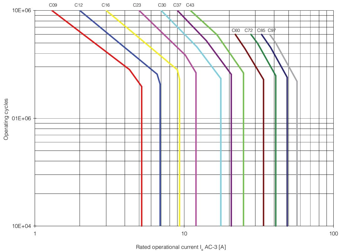
**Figure 10 - AC-4, Switching of squirrel-cage motors;  $U_e = 230\ldots690V$**
