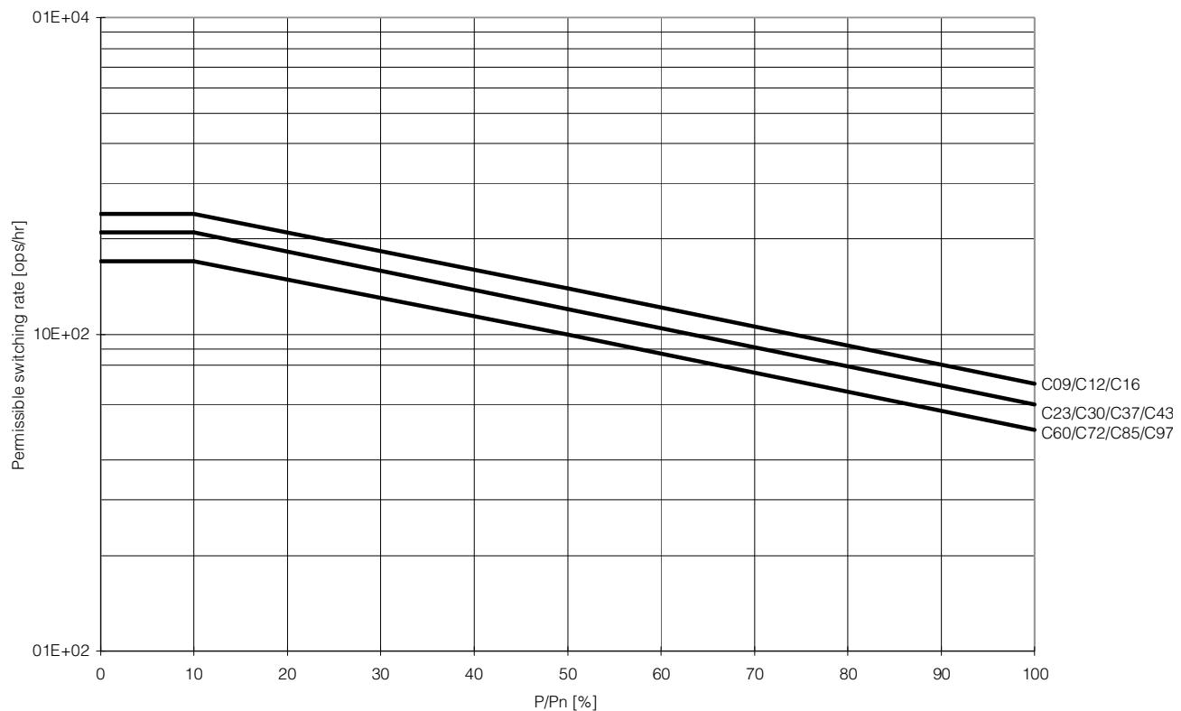
**Figure 16 - AC-4, Inching of squirrel-cage motors;  $U_e = 230\ldots460V$ , Starting time  $t_A = 0.25 s$**
