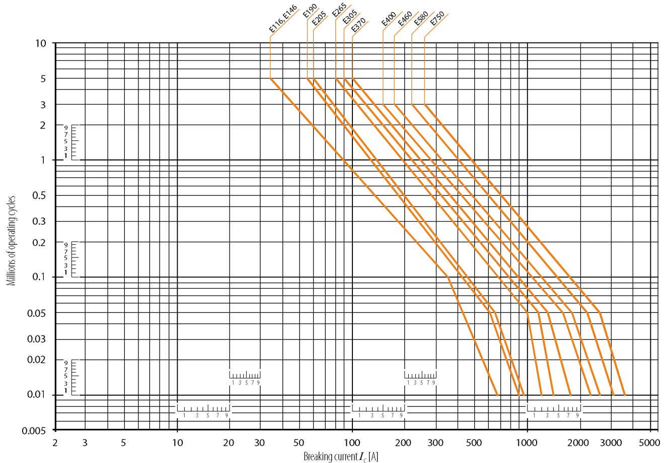
**Figure 25 - Electrical durability for AC-2 or AC-4 utilization category -  $440V < U_e \leq 690V$**
