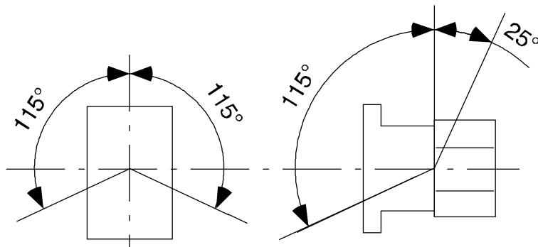
Figure 19 - Mounting Position — 100S-C DC contactors
