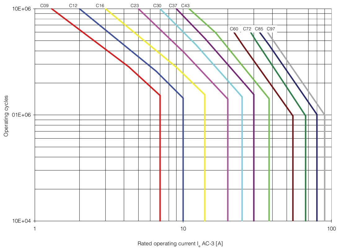
**Figure 9 - AC-3, Switching of squirrel-cage motors while starting;  $U_e = 690V$**
