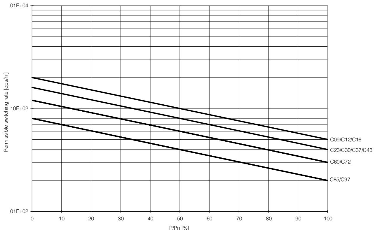
**Figure 15 - AC-3, Switching of squirrel-cage motors while starting;  $U_e = 230\ldots460V$ ; Relative operating time 40%, Starting time  $t_A = 0.25$  s**
