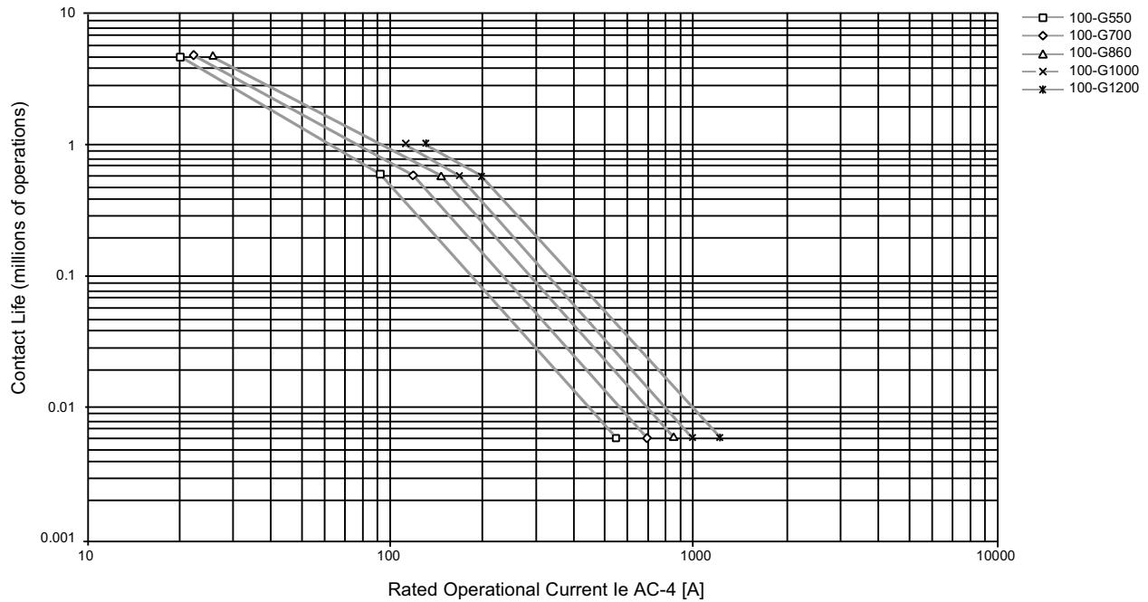
**Figure 37 - AC-3 90% Switching of Running Motors,  $U_e = 380\ldots460V$  AC; AC-4 10% Jogging**
