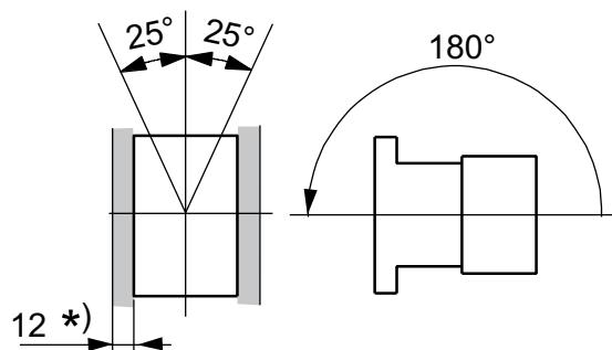
\*) -Minimum distance to grounded parts or walls
