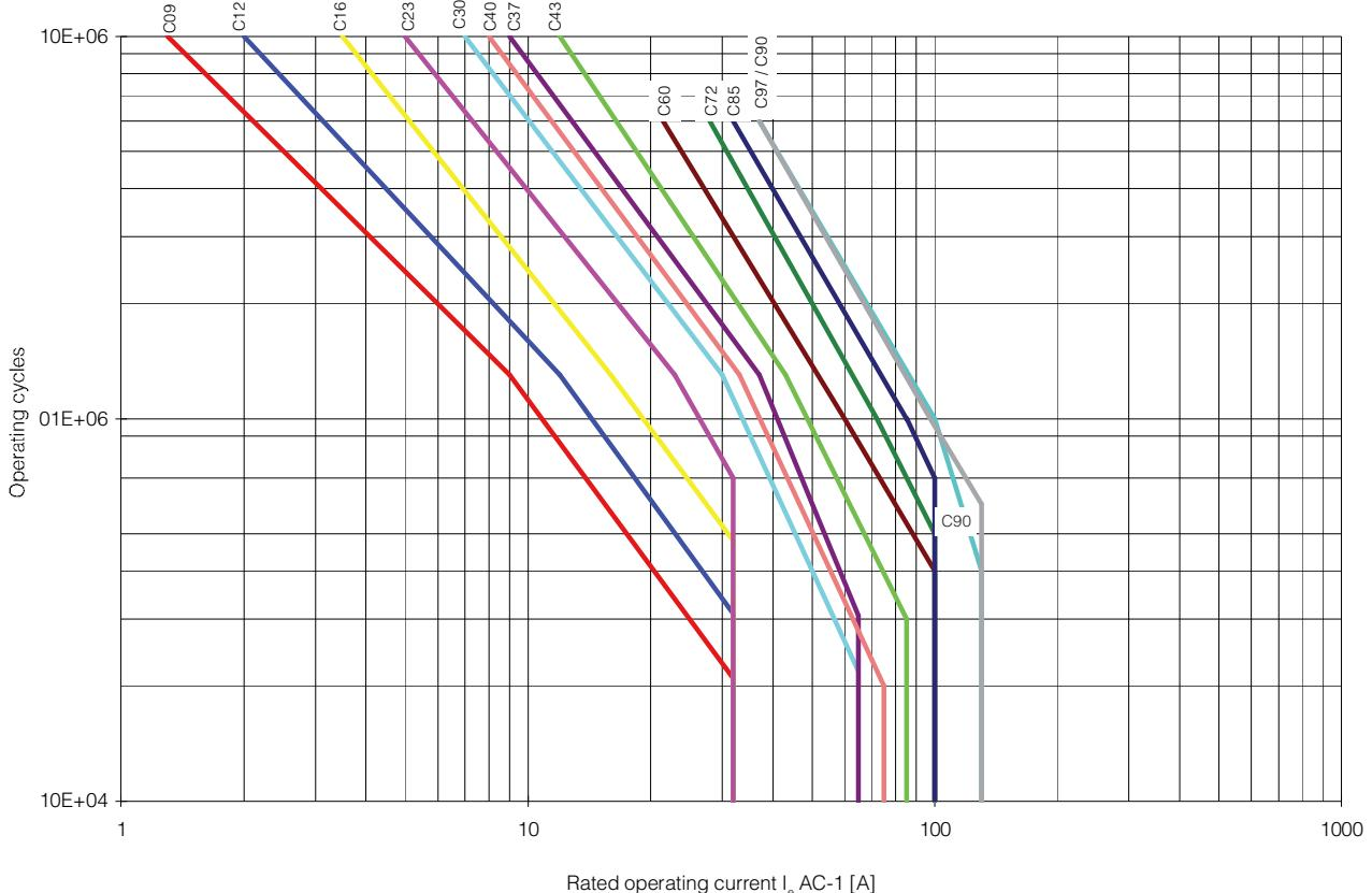
**Figure 6 - AC-2, Switching of slip-ring motors;  $U_e = 230\ldots 400\ldots 460V$**
