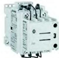
The Bulletin 100Q-C Capacitor-Switching contactors are designed for switching banks of capacitors. The unique design uses front-mounted resistor elements that limit the severely high inrush currents seen in these applications. This reduces stress to the contactors and the capacitors, as well as allowing a more compact and economical design without the use of air-core reactors.
