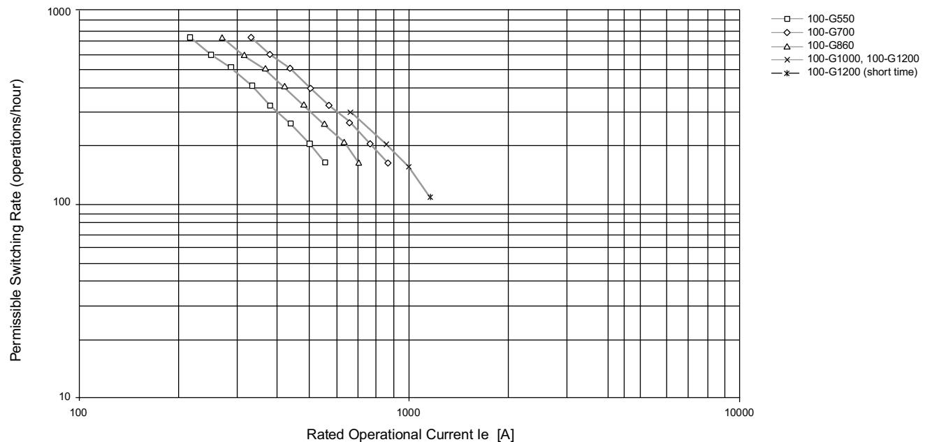
**Figure 39 - Switching of Running Squirrel-cage Motors AC-3,  $U_e = 380\ldots460V$  AC; Starting Time  $t_s = 1$  s, Relative Running Time 40%**
