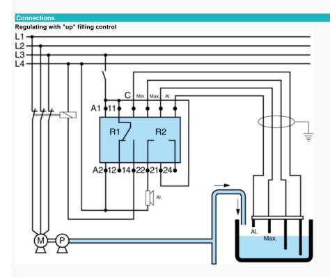
Note : In case of metalic tank, it could be used as probe (C). A green LED indicates the presence of the supply voltage A yellow LED indicates the satus of the output relay A red LED indicates the status of the alarm
