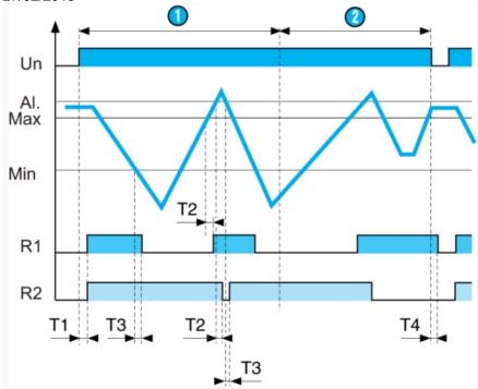
On power-up, probes Min, Max are submerged and probe AI. is above the level of the liquid. Relays R1 and R2 are energised and the pump is ON : emptying starts, the LED for relay R1 is lit. When the Min probe emerges, relay R1 de-energises and the pump if OFF : emptying stops, the LED for relay R1 goes off. If, in the event of a fault, the level continues to rise a nd reaches proble AI., relay R2 de-energises and the alarm is triggered : the LED for relay R2 is lit. This fault can be stored.
