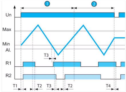
On power-up, probe AI. is submerged, relays R1 and R2 are energised and the pump is ON : filling starts, the LED for relay R1 is lit. When the level reaches the Max probe, relay R1 de-energises and the pump is OFF : filling stops, the LED for relay R1 goes off. Relay R1 re-energises when the Min probe emerges. In the event of a fault (level continues to fall) probe AI. emerges, relay R2 deenergises ans the alarme is triggered : the LED for relay R2 is lit. This fault can be stored
