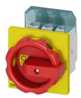
SENTRON, Switch disconnector 3LD, emergency switching-off switch, 3- pole, lu: 25 A, operating power / at AC-23 A 400 V: 9.5 kW, front-mounted, rotary operating mechanism, Red / yellow, 4-hole mounting of the handle
