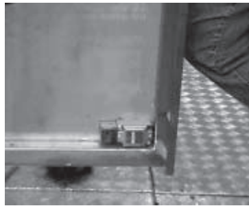
Example of a safety door interlocking system of the type series SHGV in a textiles production system.
