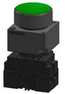
22MM METAL ROUND COMPLETE UNIT COMBINATION: ILLUMINATED PUSHBUTTON MOMENTARY CONTACT TYPE WITH FLAT BUTTON NON-ILLUMINATED WITH LAMP HOLDER BA 9S WITHOUT LAMP SCREW TERMINAL, 1NO WITH HOLDER GREEN !!! Phased-out product !!! SIRIUS ACT 3SU1 is successor Preferred successor type is >>3SU1051-0AB40-0AA0 + 3SU1550-0AA10-0AA0 + 3SU1400-1AA10-1BA0<<
