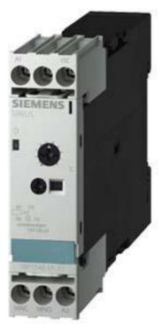
Timing relay, electronic Phased-out product !!! For further information, please contact our sales department OFF delay 1 change-over contact, without auxiliary voltage 9 time ranges, 0.05 s...600 s 24 V AC/DC with LED, Screw terminal
