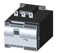
SIRIUS soft starter Values at 500 V, 40 °C standard: 313 A, 200 kW Inside-delta: 542 A, 355 kW 400-600 V AC, 230 V AC Screw terminals !!! Phased-out product !!! Successor is SIRIUS 3RW5, Preferred successor type is >>3RW5545-6HA16<<
