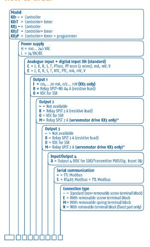
\*: For servomotor drive, both OUT2 and OUT3 codes must be selected as "M".
