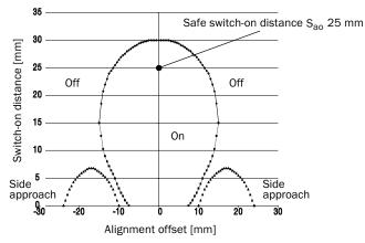
If the actuator moves laterally in relation to the surface of the sensor, a minimum distance of 7 mm must be maintained. This distance will prevent premature triggering due to the side approach areas.
