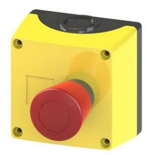
ENCLOSURE FOR COMMAND DEVICES, 22MM, ROUND, ENCLOSURE MATERIAL PLASTIC, ENCLOSURE TOP PART YELLOW, 1 COMMAND POINT, A=EMERGENCY STOP MUSHROOM PUSHBUTTON RED, 40MM, ROTATE-TO-UNLATCH, 1NC, 1NC, SCREW CONNECTION, FLOOR MOUNTING, 1 X M20 EACH AT TOP AND BOTTOM
