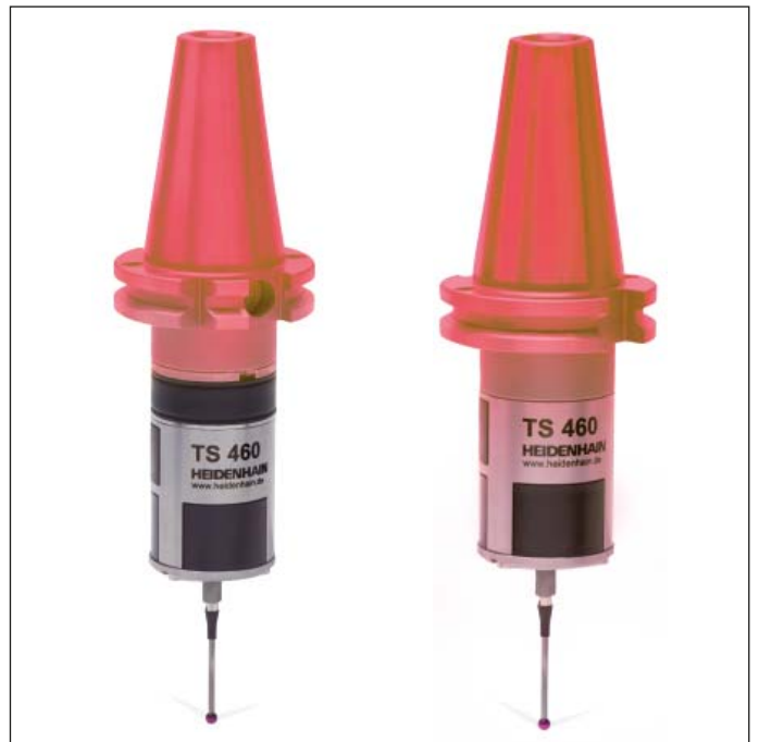
... and serves as a thermal decoupler (at left, with collision protection adapter)
