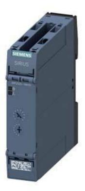
TIME RELAY, ELECTRONIC, DELAYED, 2 CO CONT., 15 TIME SET. RANGES, 0.05S...100HR, 12...240V AC/DC AT AC 50/60HZ, SCREW TERMINAL
