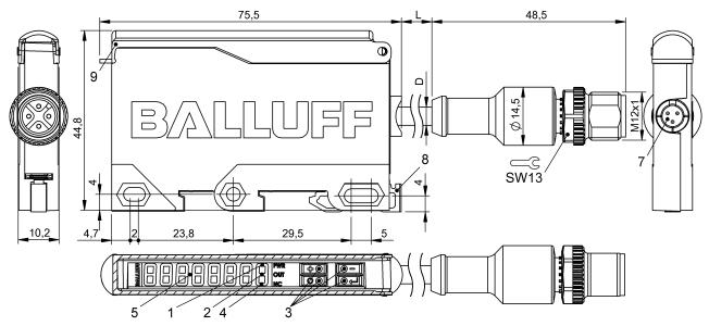
1) LED Power, 2) LED function indicator, 3) 4x operating keys, 4) LED N.C. function active, 5) 7x seven-segment display, 7) Plug connection sensor, 8) DIN rail mount 35mm, 9) Flap
