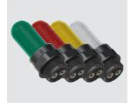
These indicator lights are used for visualizing a change of the state of an electric contact inside the switch. They can be installed only on series FL, FX, FZ, FW, FG or FS switches by screwing them on one of the conduit entries not used for electric cables, and they can have many different functions: for example, combined with a rope switch (e.g. FL 1878-M2) they can indicate (also in the distance) if the switch has been actuated.
