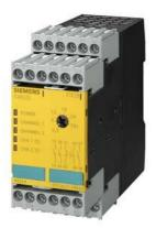
SIRIUS safety relay with relay enabling circuits (EC) 24 V DC, 45 mm overall width Screw terminal EC instantaneous: 2 NO EC delayed: 2NO, 0.5...30 s SC: 1NC AUTOSTART Basic device Maximum achieved SIL: 3/2, PL: e/d
