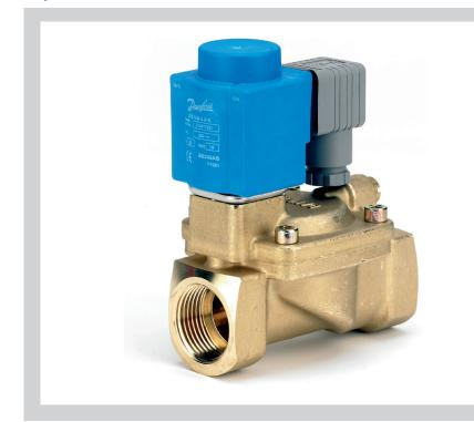
EV224B is a high pressure indirect servo-operated 2/2-way solenoid valve with working pressure up to 40 bar, medium temperature up to 60 °C and available in NC and NO versions. Built-in pilot filter as standard, replaceable equalizing orifice, enclosures up to IP67 (depending on coil) ensure a reliable and satisfactory function.
