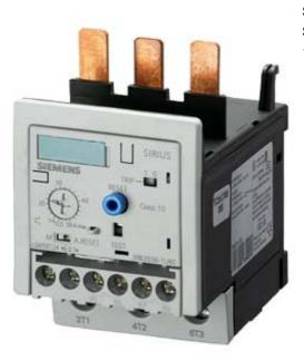
Overload relay 12.5...50 A For motor protection Size S2, Class 10 Contactor mounting Main circuit: Screw terminal Auxiliary circuit: Screw terminal Manual-Automatic-Reset !!! Phased-out product !!! Successor is SIRIUS 3RB3 Preferred successor type is >>3RB3036-1UB0<<
