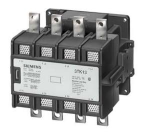
AC-1 CONTACTOR, 4-POLE, 350 A, MAIN CONTACTS 4 NO, AUXILIARY CONTACTS 2NO+2NC, AC OPERATION AC 24V 50HZ
