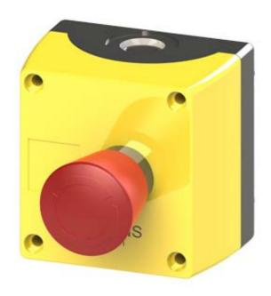
ENCLOSURE FOR COMMAND DEVICES, 22MM, ROUND, ENCLOSURE MATERIAL METAL, ENCLOSURE TOP PART YELLOW, 1 COMMAND POSITION, A=EMERG. STOP MUSHR. PUSHBUTTON RED, 40MM, ROTATE-TO-UNLATCH, 1NC, SCREW CONNECTION, FLOOR MOUNTING, 1 X M20 EACH AT TOP AND BOTTOM
