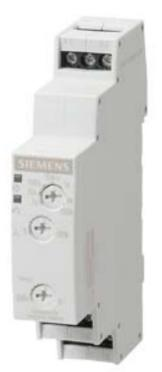
TIME RELAY, SOLID-STATE, WITH STAR-DELTA FUNCTION 2 NO 7 TIME RANGES 0.05S...100H AC/DC 12...240V SCREW TERMINAL
