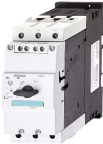
CIRCUIT-BREAKER SIZE S3 A-RELEASE 45...63A, N-RELEASE 819 A MOTOR PROTECTION, CLASS 10 SCREW CONNECTION
