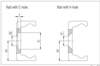
Q¹ Fixing holes for Torx® screws with low head (custom design) included in scope of supply
