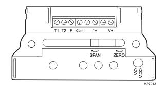
Fig. 4. Q7230A terminals and adjustments.
