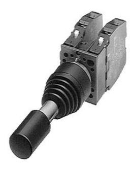
COORDINATE SWITCH, 22MM, ROUND, PLASTIC, BLACK, PLASTIC FRONT RING BLACK, 4 SWITCH POSITIONS, MOMENTARY CONTACT, WITH MECHANICAL INTERLOCK IN O POSITION, WITH HOLDER, 1NO PER DIRECTION
