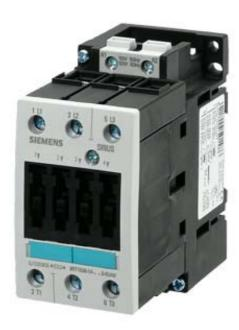
CONTACTOR, AC-3 18.5 KW/400 V, AC 24 V, 50 HZ, 3-POLE, SIZE S2, SCREW CONNECTION
