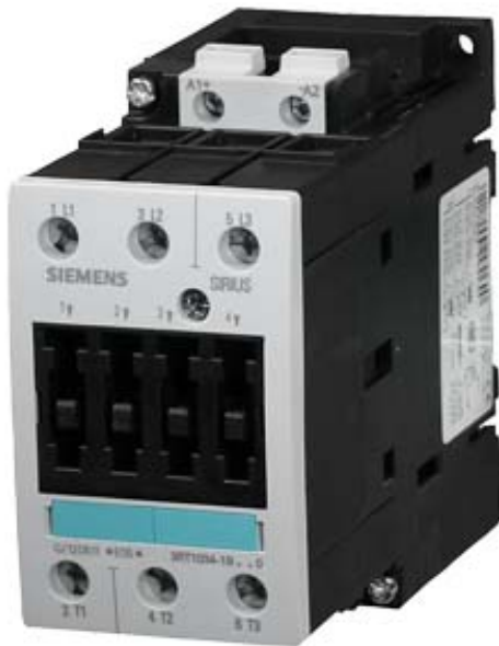
CONTACTOR, AC-3 18.5 KW/400 V, DC 24 V, 3-POLE, SIZE S2, SCREW CONNECTION
