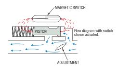
An externally rotatable vane is positioned in the main flow path within the unit. The magnet carrier piston is located in a bypass flow chamber. Pressure differential, caused by flow around the adjusting vane, displaces the spring-biased piston which actuates a hermetically sealed SPDT reed switch within the unit.
