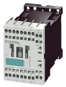
Power contactor, AC-3 7 A, 3 kW / 400 V 1 NC, 230 V AC, 50/60 Hz 3-pole, Size S00 Spring-type terminal !!! Phased-out product !!! Successor is SIRIUS 3RT2 Preferred successor type is >>3RT2015-2AP02<<
