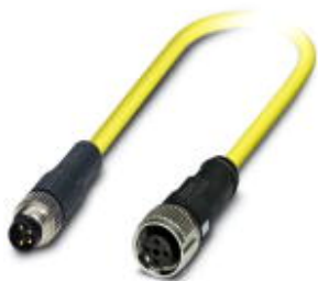
Sensor/actuator cable, 4-position, PVC, yellow, Plug straight M8, on Socket straight M12 SPEEDCON, A-coded, cable length: 1.5 m
