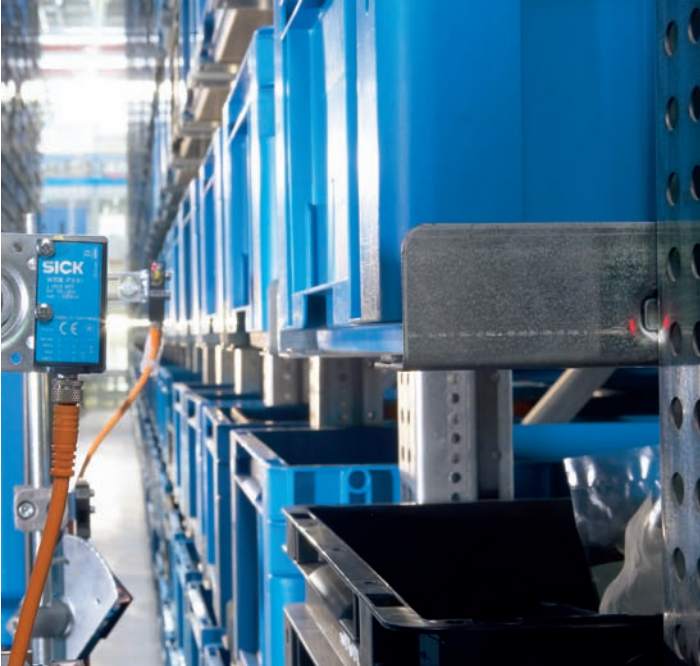
▼ ► Precise positioning of stacker cranes using the holes in the carriers.
