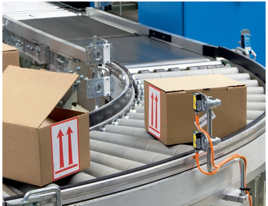
▲ Lid closed or open. An important issue for automatic wrapping. Two WL 9 lasers provide a reliable solution.
