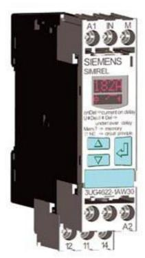
Digital monitoring relay Current monitoring, 22.5 mm from 2-500 mA AC/DC 0vershoot and undershoot 24 to 240 V AC/DC 50 to 60 Hz DC and AC ON delay and noise pulses delay 0.1 to 20 s Hysteresis 0.1 to 250 mA 1 change-over contact with or without fault buffer screw terminal Successor product for 3UG3521-1AL20, 3UG3521-1AG20 and 3UG3521-1AC48-0AA1
