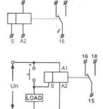
It is possible to connect load between S-A2 (e.g contactor, control of light or any other device, without disturbing a correctgunction of relay(load is energized while the switch is ON.)
